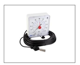
The Unitop Hydrostatic Fuel Tank Gauge is a pneumatic tank level indicator. It is designed for showing the amount of fuel oil, heating oil, diesel, bio-diesel or AdBlue™ remaining in a storage tank, it requires no power supply and is accurate to ±2 %. The Unitop Hydrostatic Fuel Tank level indicator features a spring-loaded plunging mechanism that when released causes the needle to settle on the contents left within the storage tank, which is displayed in litres.
