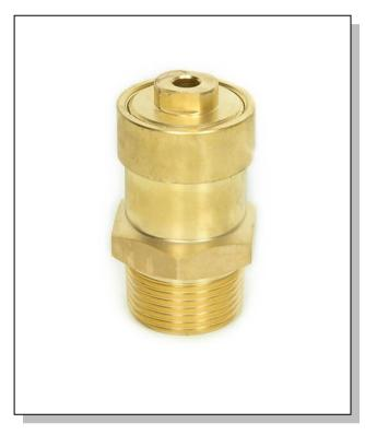
The automatic air release incorporates a floating rubber ball design feature. Air in the pipework is released through a vent hole when the system is charged with water. When the water reaches the ball chamber, the rubber ball then seats and seals the vent hole.
