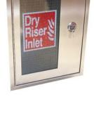
PART NUMBER:10905506 DRY RISER INLET VERTICAL MATERIAL: 16SWG ST. STEEL SATIN POLISHED BACK BOX DIMENSIONS: 595High x 395Wide x 295 Deep **MINIMUM APERTURE : 405mm** Wide x 605 High X 305 Deep
