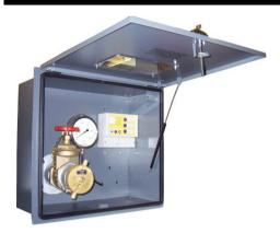
Landon Kingsway fuel fill point cabinets have been designed for filling fuel storage tanks. They are designed to be housed within the fabric of the building or built into a boundary wall. A double locking handle feature limits access to authorised personnel only. Tank levels can be read without accessing the cabinet through a polycarbonate window.
