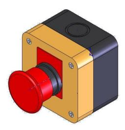
The emergency panic button has a variety of uses where it is required to have a latching push button switch to sound an alarm or isolate equipment. The switch has a normally closed contact which becomes open circuit on the switch being pressed and stays open until the button is reset.
