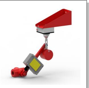
Image showing Free Fall Fire Valve arrangement with non-mercury position tilt switch with Lektro-Mag fitted on wall bracket 10901103.
